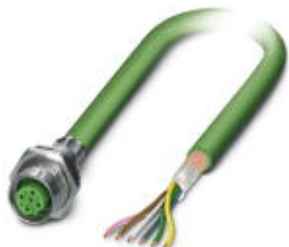
Bus system flush-type socket, INTERBUS, 5-pos., M12, shielded, B-coded, SPEEDCON, rear/screw mounting with Pg9 thread, with 5.0 m bus cable, 3 x 2 x 0.25 mm 2
