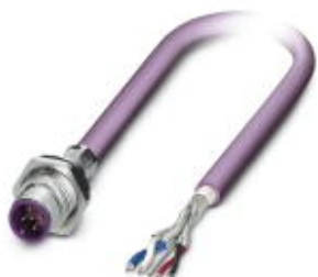
Bus system flush-type plug, DeviceNet/CANopen, 5-pos., M12, shielded, A-coded, SPEEDCON, rear/screw mounting with Pg9 thread, with 1.0 m bus cable, 2 x 0.2 mm 2 , 2 x 0.32 mm 2
