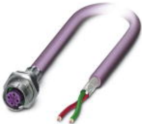
Bus system flush-type socket, PROFIBUS, 2-pos., M12, shielded, B-coded, SPEEDCON, rear/screw mounting with Pg9 thread, with 0.5 m bus cable, 2 x 0.25 mm 2
