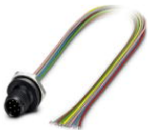
Sensor/Actuator flush-type connector, male, 8-pos., M12, A-coded, front/screw mounting with M16 thread, with 0.5 m TPE litz wire, 8 x 0.25 mm 2
