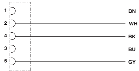
Contact assignment of the M12 socket
