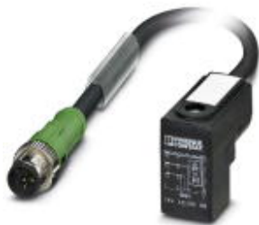
Sensor/Actuator cable, 3-position, PUR halogen-free, black-gray RAL 7021, Plug straight M12 SPEEDCON, A-coded, on Valve connector C (8 mm), with 1 LED, connected with Z diode, Cable length: 1.5 m
