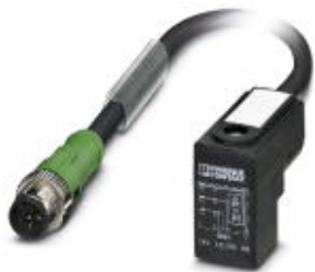
Sensor/Actuator cable, 3-position, PUR halogen-free, black-gray RAL 7021, Plug straight M12 SPEEDCON, A-coded, on Valve connector C (8 mm), with 1 LED, connected with Z diode, Cable length: 0.6 m
