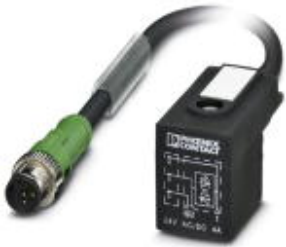
Sensor/Actuator cable, 3-position, PUR halogen-free, black-gray RAL 7021, Plug straight M12 SPEEDCON, A-coded, on Valve connector BI (11 mm), with 1 LED, connected with Z diode, Cable length: 0.3 m
