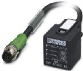
Sensor/Actuator cable, 3-position, PUR halogen-free, black-gray RAL 7021, Plug straight M12 SPEEDCON, A-coded, on Valve connector A, with 1 LED, connected with Z diode, Cable length: 0.6 m
