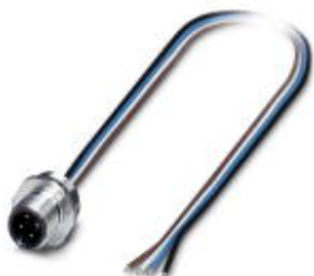
Bus system flush-type connector, FOUNDATION Fieldbus, plug, 4-pos., M12, A-coded, front/screw mounting with Pg9 thread, with 0.5 m TPE litz wire, 3 x 0.34 mm², stainless steel version
