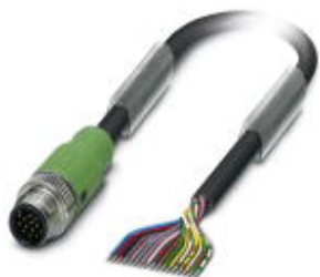
Sensor/Actuator cable, 17-position, PUR halogen-free, black RAL 9005, Plug straight M12 SPEEDCON, A-coded, on free cable end, Cable length: 1.5 m
