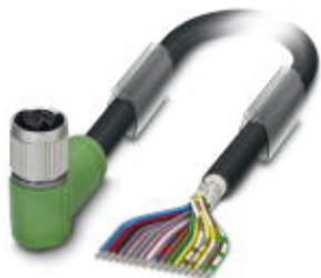
Sensor/Actuator cable, 17-position, PUR/PVC, black RAL 9005, shielded, free cable end, on Socket angled M12 SPEEDCON, A-coded, Cable length: 10 m
