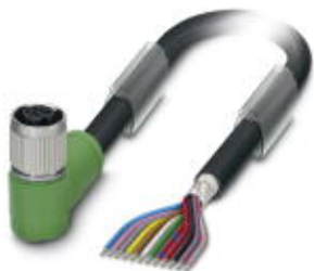
Sensor/Actuator cable, 12-position, PUR/PVC, black RAL 9005, shielded, free cable end, on Socket angled M12 SPEEDCON, A-coded, Cable length: 3 m
