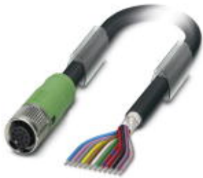
Sensor/Actuator cable, 12-position, PUR/PVC, black RAL 9005, shielded, free cable end, on Socket straight M12 SPEEDCON, A-coded, Cable length: 1.5 m
