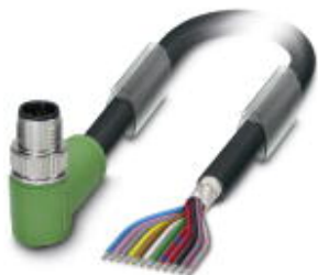
Sensor/Actuator cable, 12-position, PUR/PVC, black RAL 9005, shielded, Plug angled M12 SPEEDCON, A-coded, on free cable end, Cable length: 3 m
