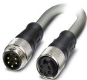
Power cable, 5-position, PUR, gray RAL 7001, Plug straight 7/8"-16UNF, A-coded, on Socket straight 7/8"-16UNF, A-coded, Cable length: 2 m, 2.5 mm 2 conductor cross section, For power supply
