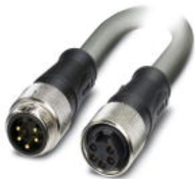
Power cable, 5-position, PUR, gray RAL 7001, Plug straight 7/8"-16UNF, A-coded, on Socket straight 7/8"-16UNF, A-coded, Cable length: 1.5 m, 2.5 mm 2 conductor cross section, For power supply
