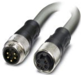
Power cable, 5-position, PUR, gray RAL 7001, Plug straight 7/8"-16UNF, A-coded, on Socket straight 7/8"-16UNF, A-coded, Cable length: 0.6 m, 2.5 mm 2 conductor cross section, For power supply
