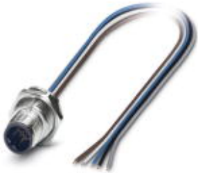
Sensor/actuator flush-type plug, 5-pos., M12 SPEEDCON, B-coded, rear/screw mounting with M16 thread, with 0.5 m TPE litz wire, 5 x 0.34 mm 2
