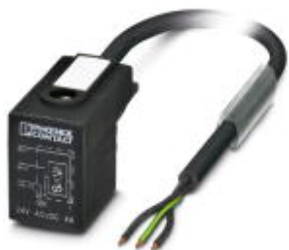
Sensor/Actuator cable, 3-position, PVC, black RAL 9005, free cable end, on Valve connector BI (11 mm), with 1 LED, connected with Varistor, Cable length: 3 m
