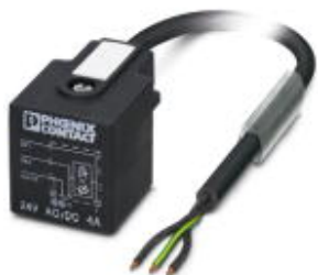
Sensor/Actuator cable, 3-position, PVC, black RAL 9005, free cable end, on Valve connector A, with 1 LED, connected with Varistor, Cable length: 10 m
