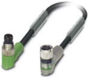
Sensor/Actuator cable, 3-position, PVC, black RAL 9005, Plug angled M8, on Socket angled M8, with 2 LEDs, Cable length: 3 m
