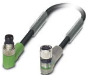
Sensor/Actuator cable, 3-position, PVC, black RAL 9005, Plug angled M8, on Socket angled M8, with 2 LEDs, Cable length: 0.3 m
