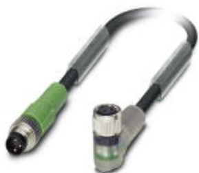
Sensor/Actuator cable, 3-position, PVC, black RAL 9005, Plug straight M8, on Socket angled M8, with 2 LEDs, Cable length: 0.3 m
