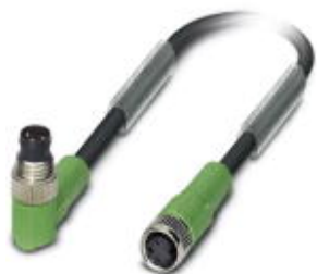
Sensor/Actuator cable, 3-position, PVC, black RAL 9005, Plug angled M8, on Socket straight M8, Cable length: 0.6 m
