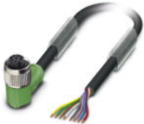
Sensor/Actuator cable, 8-position, PVC, black RAL 9005, free cable end, on Socket angled M12, A-coded, Cable length: 10 m
