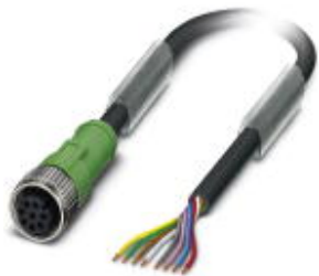
Sensor/Actuator cable, 8-position, PVC, black RAL 9005, free cable end, on Socket straight M12, A-coded, Cable length: 10 m
