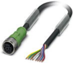
Sensor/Actuator cable, 8-position, PVC, black RAL 9005, free cable end, on Socket straight M12, A-coded, Cable length: 5 m
