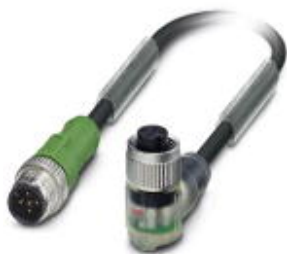
Sensor/Actuator cable, 5-position, PVC, black RAL 9005, Plug straight M12, A-coded, on Socket angled M12, A-coded, with 3 LEDs, Cable length: 0.3 m
