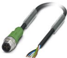
Sensor/Actuator cable, 5-position, PVC, black RAL 9005, Plug straight M12, A-coded, on free cable end, Cable length: 3 m
