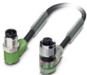
Sensor/Actuator cable, 4-position, PVC, black RAL 9005, Plug angled M12, A-coded, on Socket angled M12, A-coded, with 3 LEDs, Cable length: 1.5 m
