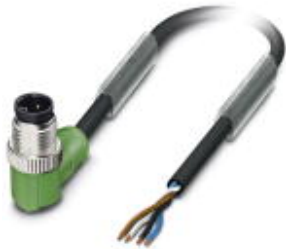
Sensor/Actuator cable, 4-position, PVC, black RAL 9005, Plug angled M12, A-coded, on free cable end, Cable length: 1.5 m
