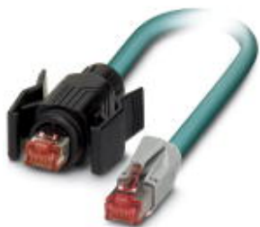
Assembled Ethernet cable, CAT6, shielded, 4-pair, AWG 26 stranded (7-wire), RAL 5021 (water blue), RJ45 plug/IP67, black on RJ45 plug/IP20, line, length 5 m
