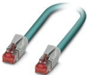
Assembled Ethernet cable, CAT6, shielded, 4-pair, AWG 26 stranded (7-wire), RAL 5021 (water blue), RJ45 plug/IP20 on RJ45 plug/IP20, line, length 2 m
