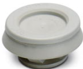
Membrane screw connection, Cable gland material: Polypropylene, Application: Standard, External cable diameter 4 mm ... 10 mm, Shielding: No, Connecting thread: M16, Color: lightgrey RAL 7035
