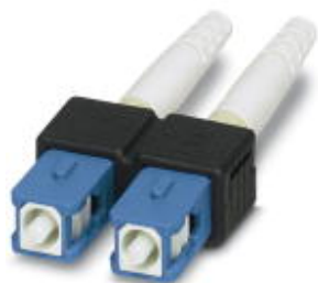
SC duplex connector, with long bend protection, for single mode 9/125 µm, PC polishing, blue, value pack: 10 pcs
