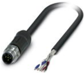
Bus system cable, CANopen®, DeviceNet™, 5-position, FRNC halogen-free, black, shielded, Plug straight M12, A-coded, on free cable end, Cable length: 2 m, for outdoor applications, With high-grade steel knurl
