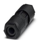
QUICKON cable connector, black, 4+PE-pos., 2.5 mm<sup>2</sup> ... 6.0 mm<sup>2</sup>/690 V/40 A, for cable diameter of 12 mm ... 20 mm.
