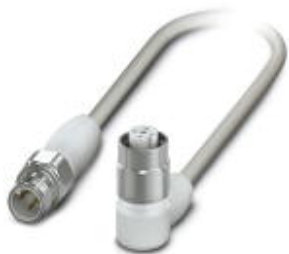
Sensor/Actuator cable, 4-position, PP-EPDM halogen-free, gray RAL 7035, Plug straight M12, A-coded, on Socket angled M12, A-coded, Cable length: 0.3 m, Hygienic design, With high-grade steel knurl
