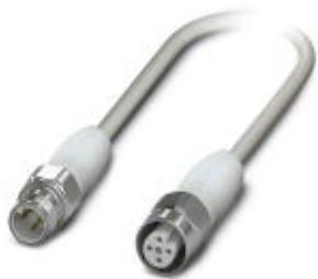
Sensor/Actuator cable, 4-position, PP-EPDM halogen-free, gray RAL 7035, Plug straight M12, A-coded, on Socket straight M12, A-coded, Cable length: 3 m, Hygienic design, With high-grade steel knurl
