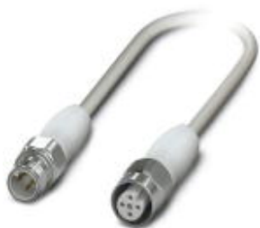
Sensor/Actuator cable, 4-position, PP-EPDM halogen-free, gray RAL 7035, Plug straight M12, A-coded, on Socket straight M12, A-coded, Cable length: 0.3 m, Hygienic design, With high-grade steel knurl
