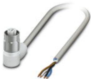
Sensor/Actuator cable, 4-position, PP-EPDM halogen-free, gray RAL 7035, free cable end, on Socket angled M12, A-coded, with 3 LEDs, Cable length: 10 m, Hygienic design, With high-grade steel knurl
