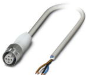
Sensor/Actuator cable, 4-position, PP-EPDM halogen-free, gray RAL 7035, free cable end, on Socket straight M12, A-coded, Cable length: 10 m, Hygienic design, With high-grade steel knurl
