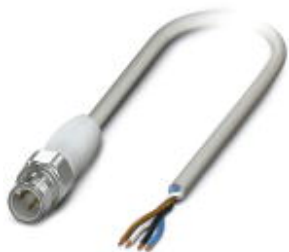
Sensor/Actuator cable, 4-position, PP-EPDM halogen-free, gray RAL 7035, Plug straight M12, A-coded, on free cable end, Cable length: 1.5 m, Hygienic design, With high-grade steel knurl
