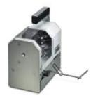
Automatic stripping and crimping device, 120 V version, for insulated taped ferrules  $0.5 - 2.5 \text{ mm}^2$  in acc. with DIN 46228-4: 1990-10
