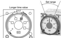
Note) The stoppers for the lower limit setting set ring and the upper limit setting set ring face the opposite directions.
