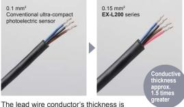
increased to 0.15 mm<sup>2</sup> from 0.1 mm<sup>2</sup> of the conventional ultra-compact photoelectric sensor. This makes it easier to perform crimpling work on the cables for better workability. In addition, the tensile strength of the crimpling area has become stronger.
