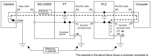
\*The example in the above figure shows a computer connected to an RS-232C connector on the PLC.
