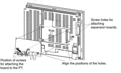
(2) Push firmly on the connector end of the board and make sure that it is inserted sufficiently.
