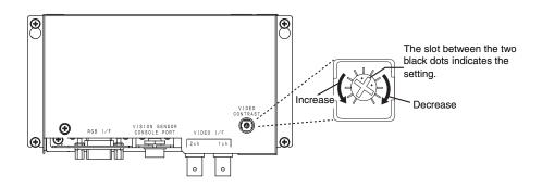
\* The image may be distorted if the contrast adjustor is turned too far. When that happens, turn the adjustor in the opposite direction until the distortion is eliminated.
