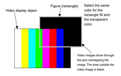
Select **PT - System Setting** on the CX-Designer, and then set the *Color which fills blank channels* field from the System Setting Dialog Box that is displayed.
