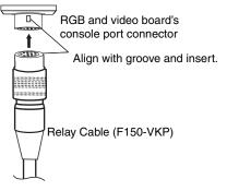
The socket locks into place when it is inserted.
