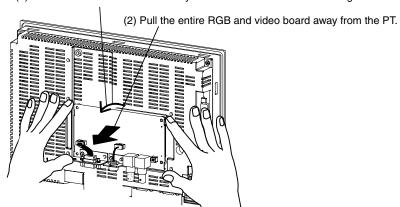
(1) Hold the RGB and video board by the corners and remove it starting from the top.
