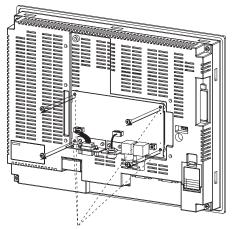
Remove the screws securing the four corners.
