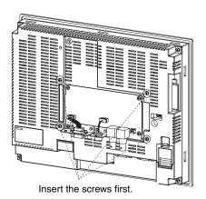
(5) Align the cover screw holes with the screws and mount the cover.
