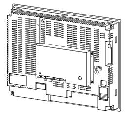
(6) Slide the cover downward and tighten the screws.
