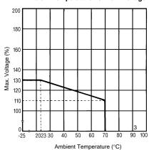
NOTE: The maximum voltage is the permissable peak voltage that can be imposed on the coil The maximum voltage must not be imposed on the coil continuously.
