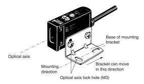
Note: The maximum tightening torque applied to the screw is 5.5 kgf x cm (0.53 N x m).
