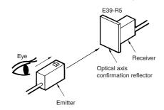
Attach the reflector to the receiver (refer to the figure). Look at the reflector from right behind the emitter. The reflector should be bright with red light when the optical beam strikes the reflector. If the emitter has a turbo function, the reflector looks brighter with the function switched on.
