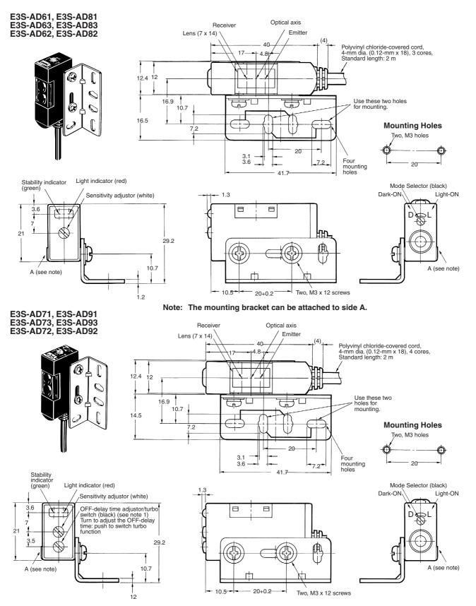
Note: 1. Turbo switch is only for E3S-AD71 and E3S-AD91. 2. The mounting bracket can be attached to side A.
