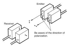
The arrow printed on the cover indicates the direction of polarization. By attaching the filters opposite to each other in polarization to the emitters and the receivers (refer to the figure) in rows, mutual interference can be prevented (in any case, the filter attached to an emitter and to the corresponding receiver must be the same in direction of polarization or the photoelectric sensor will not function).
