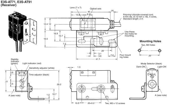
Note: The mounting bracket can be attached to side A.
