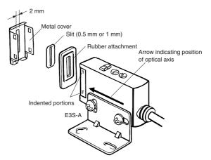
Note: Apply the slit to the lens of the photoelectric sensor marked with an arrow indicating the position of the optical axis (apply it to the bottom lens of horizontal sensors and the top lens of vertical sensors).
