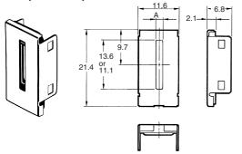
Note: The width of A is 0.5 mm, 1 mm, or 2 mm depending on the model.
