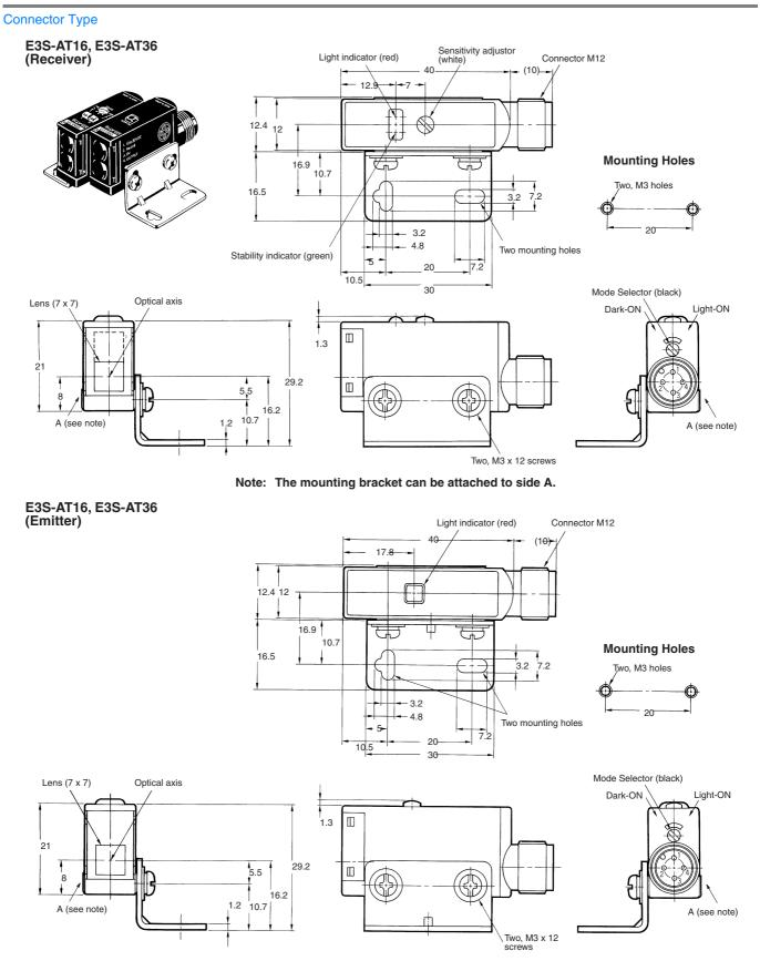
Note: The mounting bracket can be attached to side A.
