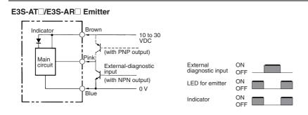
The sensor is normal if the control output varies when the self-diagnostic external input is ON and OFF. The sensor is abnormal if the control output does not vary when the self-diagnostic external input is turned ON or OFF.
